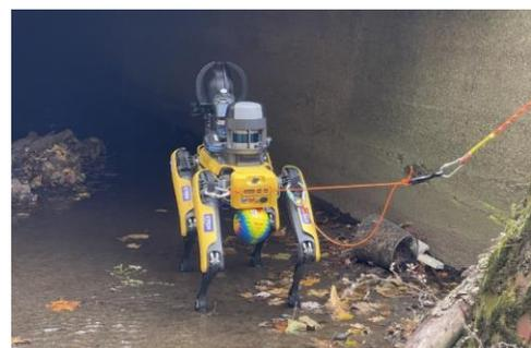
Figure 6. Mudge the robotic sampling "dog" entering a confined space culvert underneath East Palestine.
