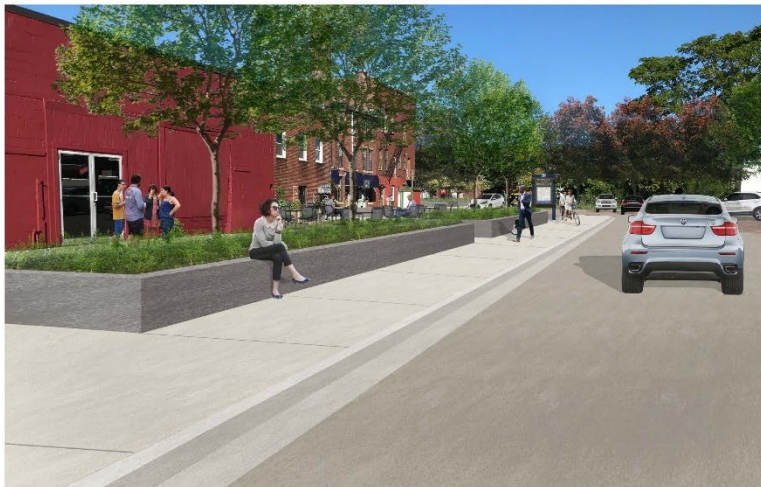
Figure 13: Design concept for public parking lot. The perspective shows an expanded pedestrian area behind North Main Street businesses with granite above ground planters, shade trees, a pervious paver courtyard, wayfinding signage, pervious paver parking spaces, and enhanced vegetation screening along Union Street.
