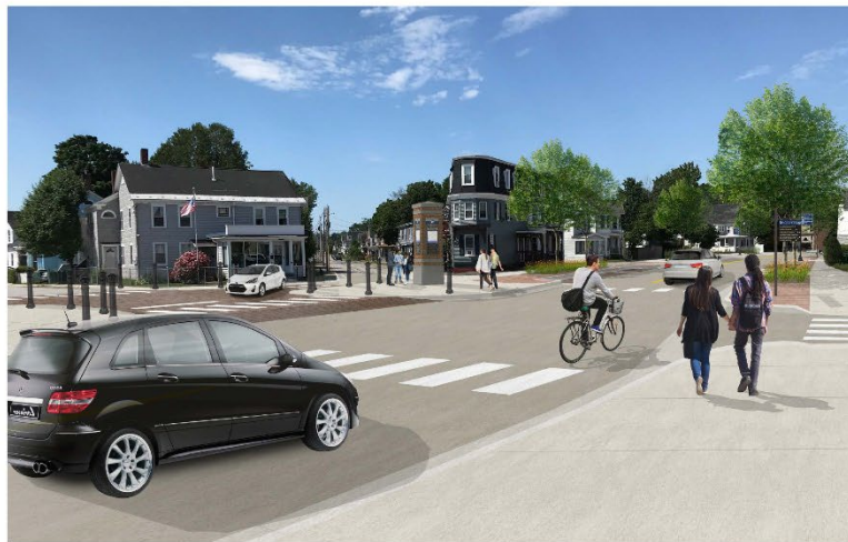
Figure 6: Design concept for North Main Street. The perspective shows two lanes of traffic with shared use lanes, a reconfigured River Street and Pine Street intersection as a pervious paver tabletop, a neighborhood monument, pervious paver parallel parking spaces, stormwater planters, splash guard behind curb, historic lighting and wayfinding signage.
