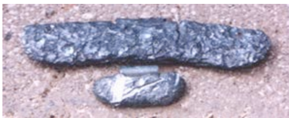
Figure 8: An example of wheel weight abrasion. Notice the deformity when compared to the weights in Figure 6.
