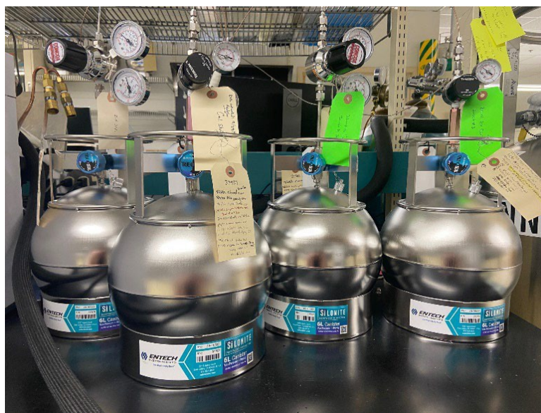
Figure 4. Internal standard canister (first on left), calibration standard canister (second from left), SSCV canister (third from left), and method blank canister (far right) installed on Entech 7200A.
