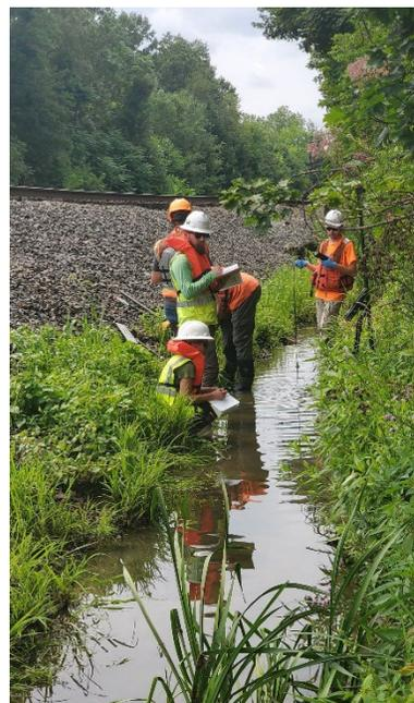
*Figure 6. Initial sediment investigations have been conducted in Sulphur Run and Leslie Run which indicated that some contamination from the derailment remains which causes a sheen on the surface water when sediments are disturbed.*
