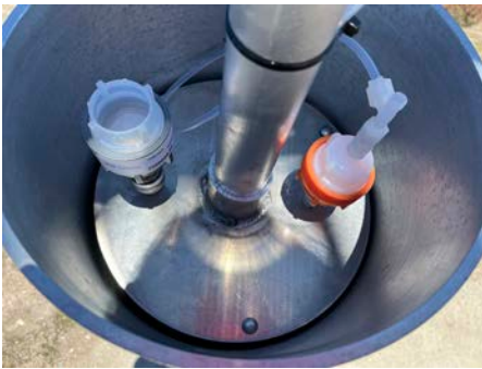
Close up of the thermos science 49i O3 filter pack.
