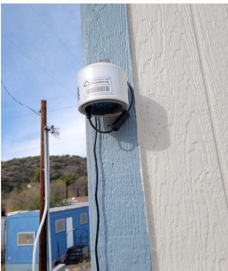
A PurpleAir sensor monitoring ambient air quality outside a La Jolla Band building.
