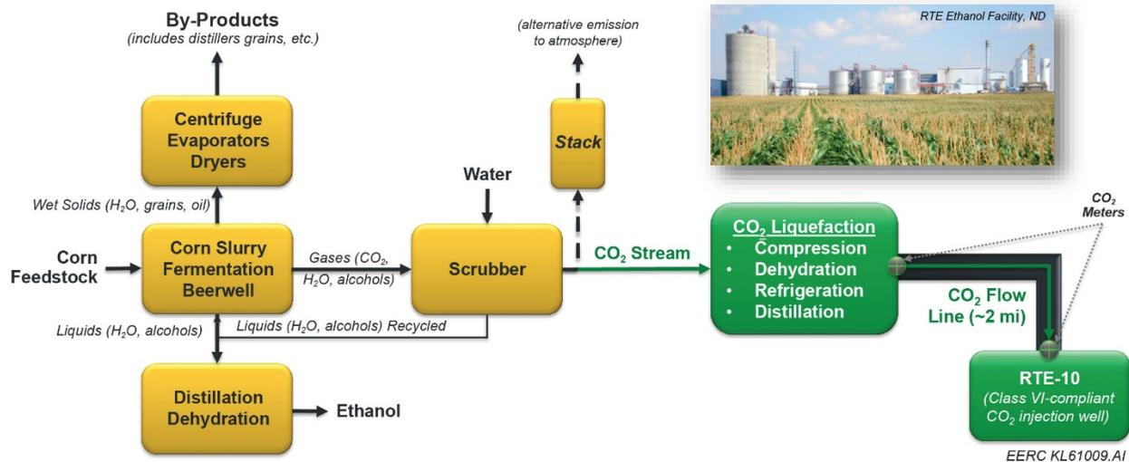
Figure 1-4. Flow diagram of the RTE CCS process, showing major CCS components and the path of the CO<sub>2</sub> stream from the capture facility to the RTE-10 injection well.
