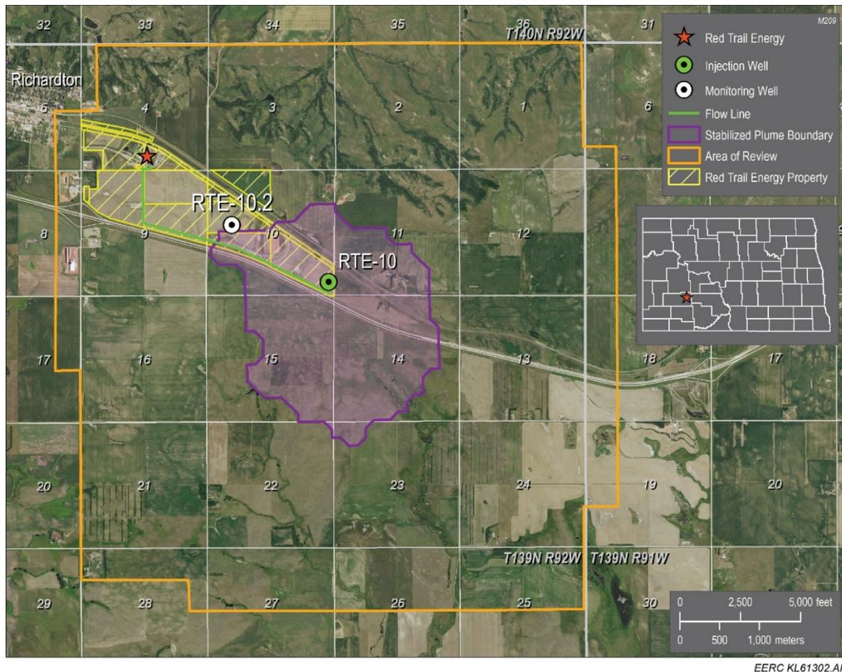
Figure 1-1. Location of the RTE facility, RTE-10 injection well, RTE-10.2 monitoring well, and CO<sub>2</sub> flowline. Also shown is the town of Richardton, with a population of about 850 people, the stabilized plume boundary, and the area of review (AOR).
