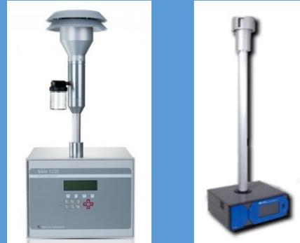
The Federal Equivalent Methods (FEMs) provide automated data at higher time resolution (generally every hour). They are used across the official air monitoring network and were designated by comparison to FRMs under typical conditions (not smoke).
