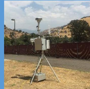
Temporary monitors also provide hourly data, were tested for performance under high concentrations, and are used extensively by government organizations for supplemental monitoring during wildland fire smoke events.
