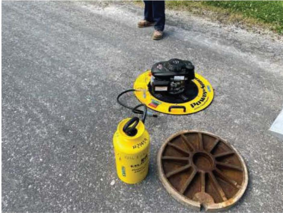
Sanitary sewer smoke testing equipment
