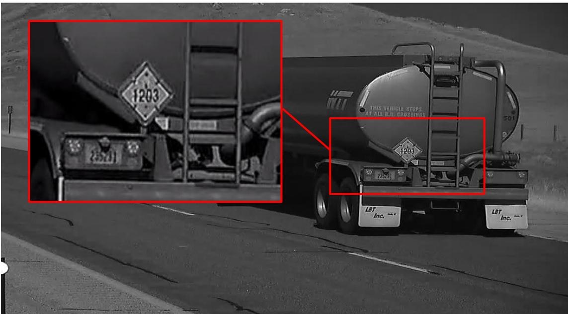
a) Image from the LPR camera pointed at the placards mounted at the back
