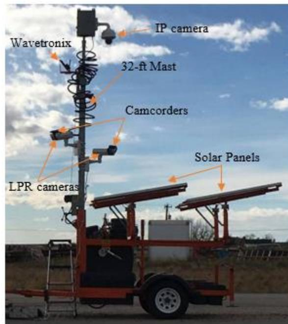
**Figure 21: HAZMAT data collection trailer**
