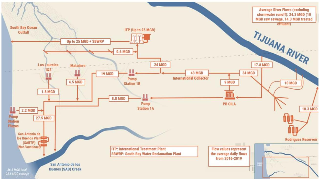
**Figure 2-3** Lift stations locations near the border.
