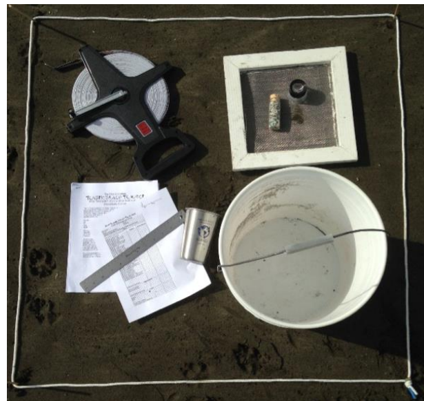
Figure 2. Clockwise from upper left: Tape measure, sieve with magnifying glass and glass bottles, bucket, metal cup, ruler and data sheets, all within the 1 x 1-meter quadrat.
