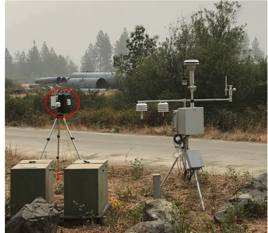
Air sensors (red circle) collocated with a temporary smoke monitor during the Natchez Fire (Happy Camp, CA)
