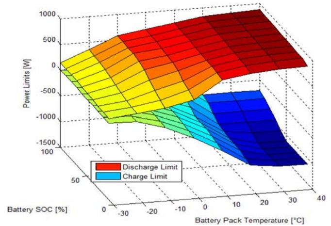
Figure 3. Averaged Discharge and Charge Power Limit Surfaces of a Lithium Iron-Phosphate Battery Cell
