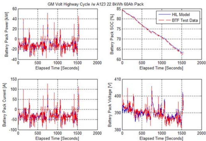
Figure 15. GM Volt Pack Voltage, Current, SOC HIL Simulations in 2 x Highway Drive Cycles
