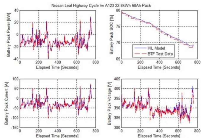
Figure 11. Battery voltage, Current and SOC of Nissan Leaf Pack Emulation during Highway Drive Cycle
