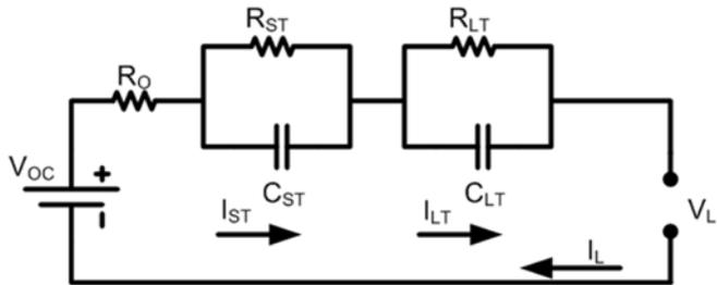
Figure 1. Battery Equivalent Circuit Cell Model
