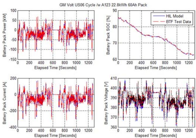
Figure 16. GM Volt Pack Voltage, Current, SOC HIL Simulations in 2 x US06 Drive Cycles
