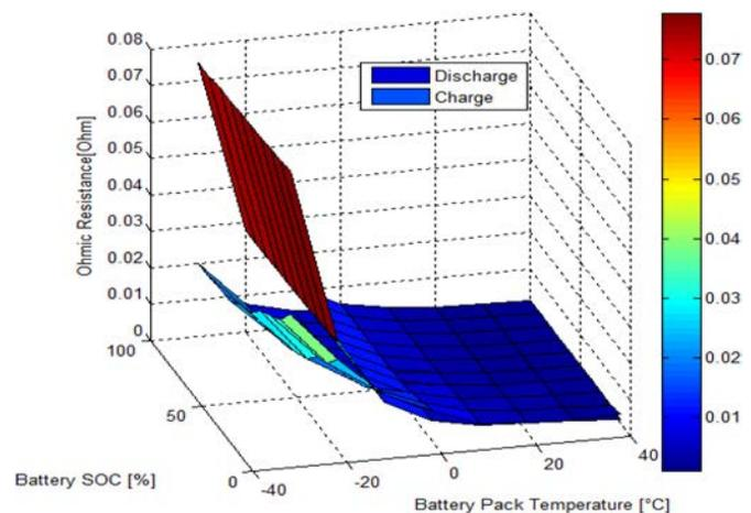
Figure 5. Averaged Discharge and Charge Resistance Surfaces of Lithium-Ion Battery Cells
