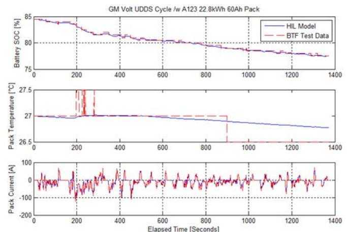
Figure 14. Battery SOC, Pack Voltage of GM Volt Pack Emulation during UDDS Cycle
