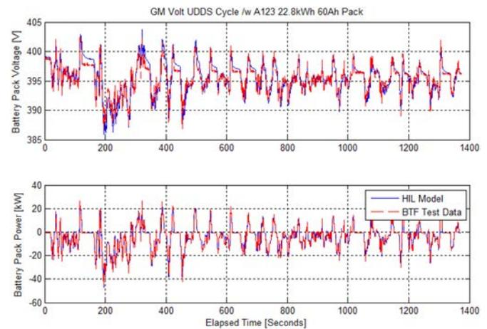
Figure 13. Battery Pack Voltage of GM Volt Pack Emulation during UDDS Cycle
