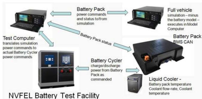
Figure 6. EPA NVFEL Battery Test Facility Hardware-In-Loop (HIL)
