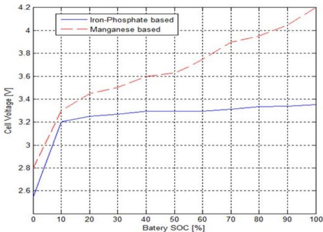
Figure 2. Typical Open Circuit Voltage (OCV) of Lithium-Ion Battery Cells
