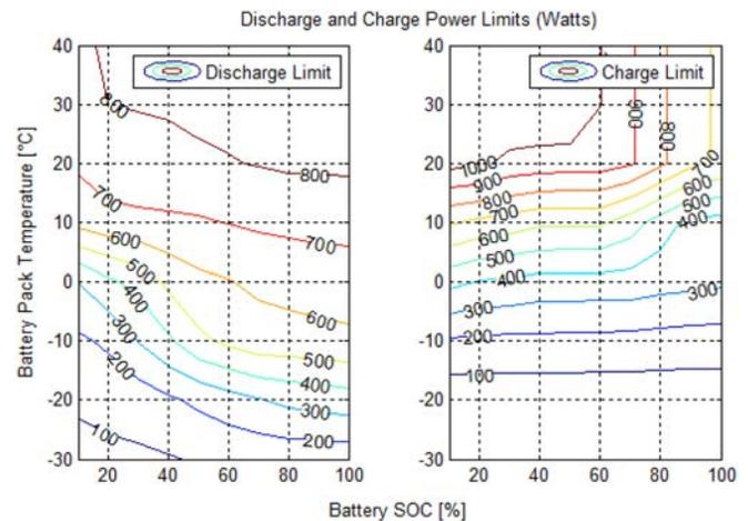
Figure 4. Averaged Discharge and Charge Power Limit Contour Plots of a Lithium Iron-Phosphate Battery Cell
