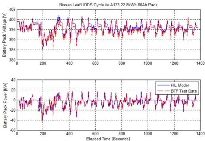
Figure 9. Battery Pack Voltage of Nissan Leaf Emulation during UDDS Cycle
