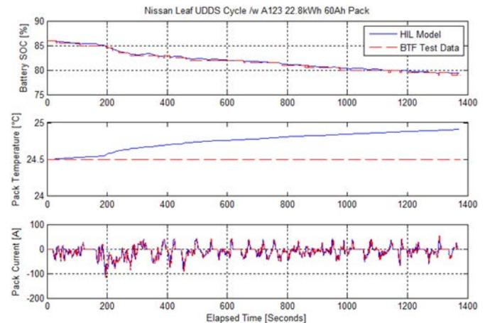
Figure 10. Battery Pack SOC and temperature of Nissan Leaf Pack Emulation during UDDS Cycle
