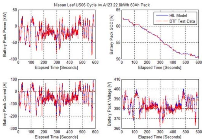
Figure 12. Battery voltage, Current and SOC of Nissan Leaf Pack Emulation during US06 Drive Cycle
