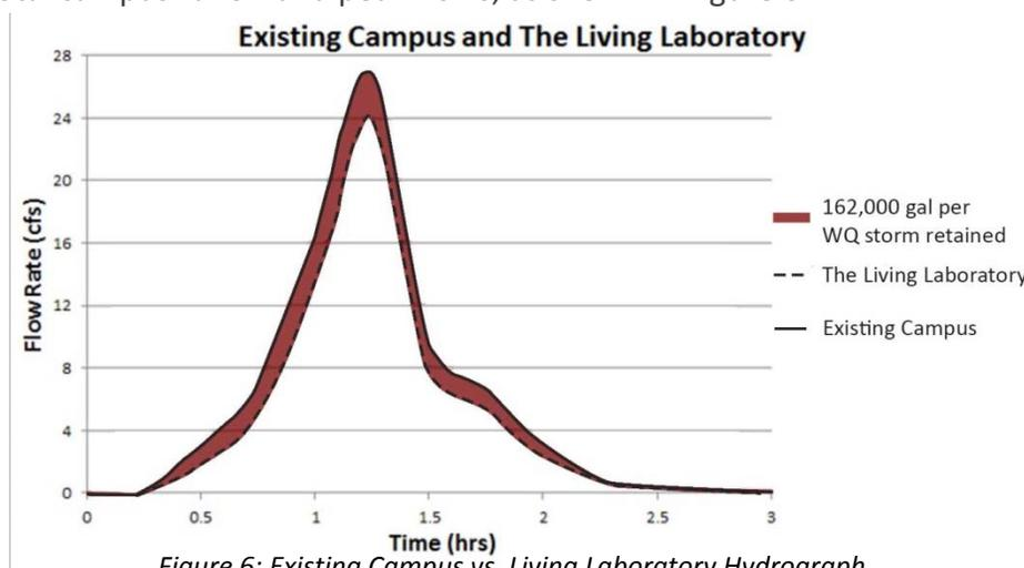
The introduction of GI to the Stevens campus results in a 10.5% reduction (2.83 cfs) in peak flow of stormwater leaving the campus. The Living Laboratory will capture 0.162 MG during each WQ storm, a 20% reduction in runoff from the current conditions on campus.
