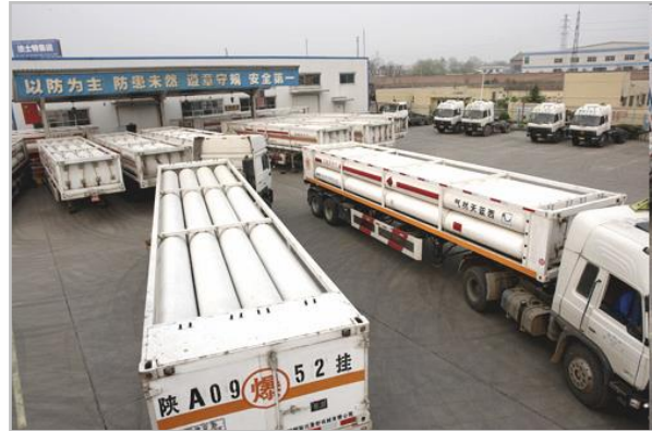
Exhibit 5-11: CNG Transport Trucks
