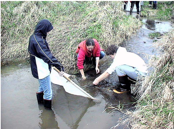
Students disturb the stream bottom to knock benthic macroinvertebrates into the water column, where they are carried downstream and captured in a kick seine net. Students first use their hands to rub rocks on the stream bottom (as seen above). Next, they will “kick around” in the stream bottom to dislodge additional macroinvertebrates hiding in the substrate.
