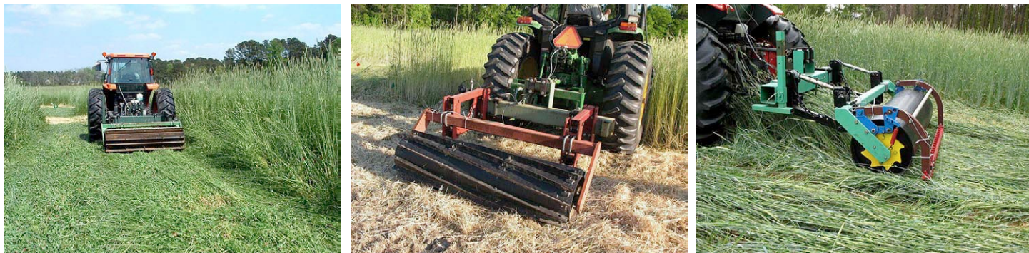
Roller designs may include straight horizontal crimping bars (left photo), curved crimping bars (middle photo), or a smooth drum attached to a single crimping bar (right photo). (Photos by Ted Kornecki)
