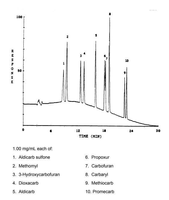
This chromatogram was produced using the instrument operating conditions described in Sec. 7 and is for illustrative purposes only.
