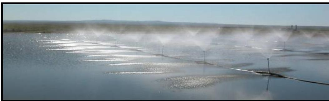
**Figure 4: Sprays Used to Enhance Evaporation**
